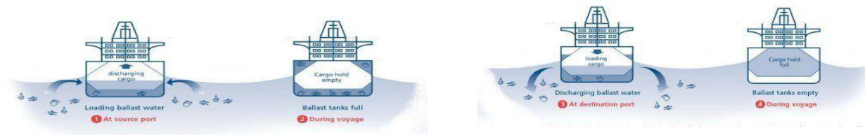
The loading of ballast water. (Image courtesy of the international Maritime Organization)
